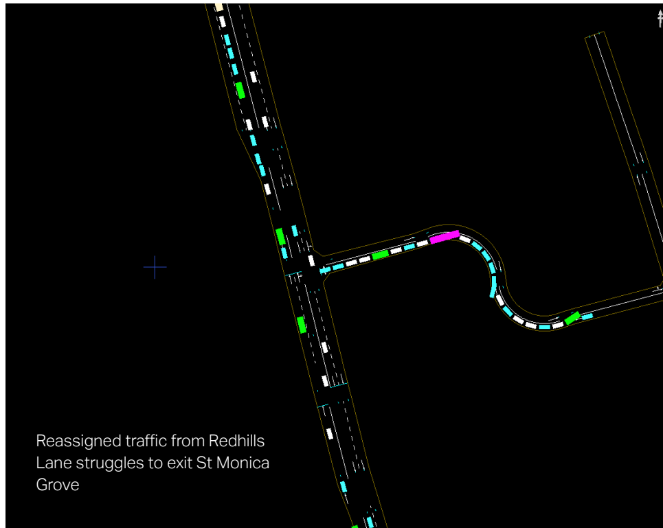
Figure 4-5: Queueing on St Monica Grove as a Result of Proposed Scheme
