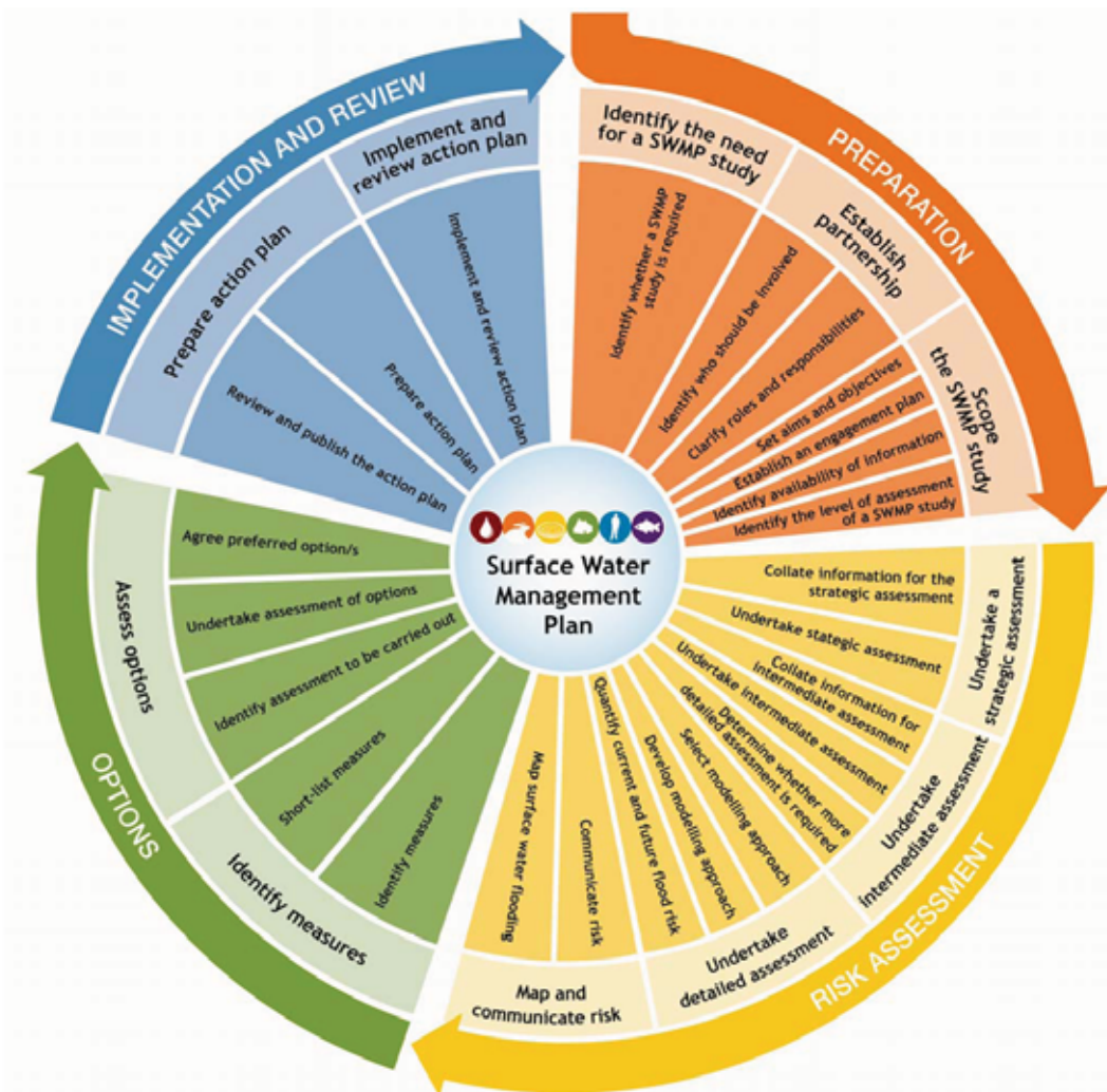
Figure C.1.2: SWMP Process (Defra 2010)
